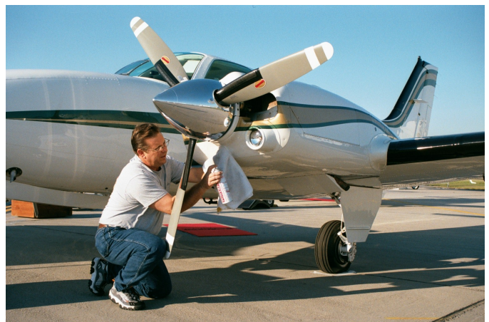
24 Using Powerfoam to clean bugs and oil from Barron B-58 engine cowling.
