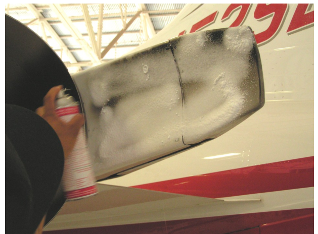
Powerfoam removing carbon from exhaust deflector at the rear of Hawker 1000.
