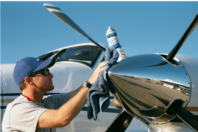
Use Plexi-Clear or Quick Turn to clean polished aluminum spinner on King Air 200.
