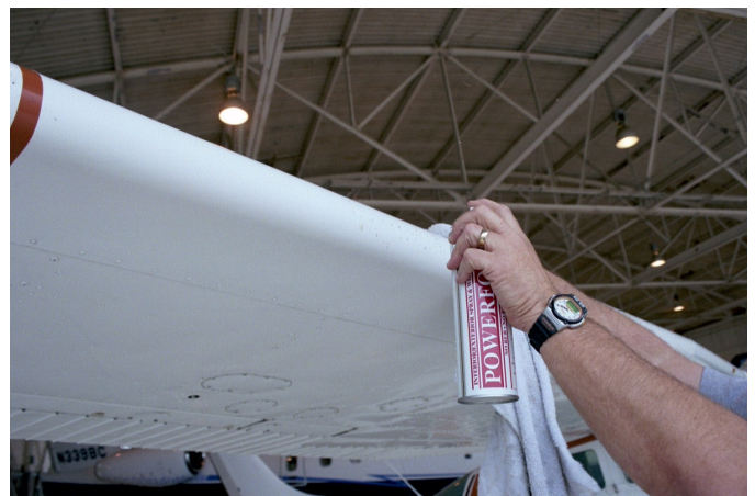
Use Powerfoam or Quick-Turn to clean bugs from leading edges of Cessna 206.
