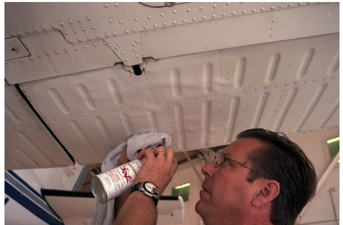
Using Powerfoam to clean bugs off bottom of flap on Cessna 206.
