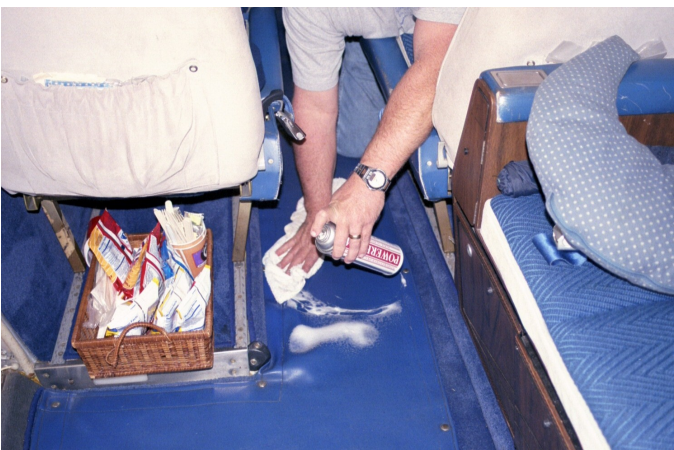
Using Powerfoam to clean floor runners in King Air 200
