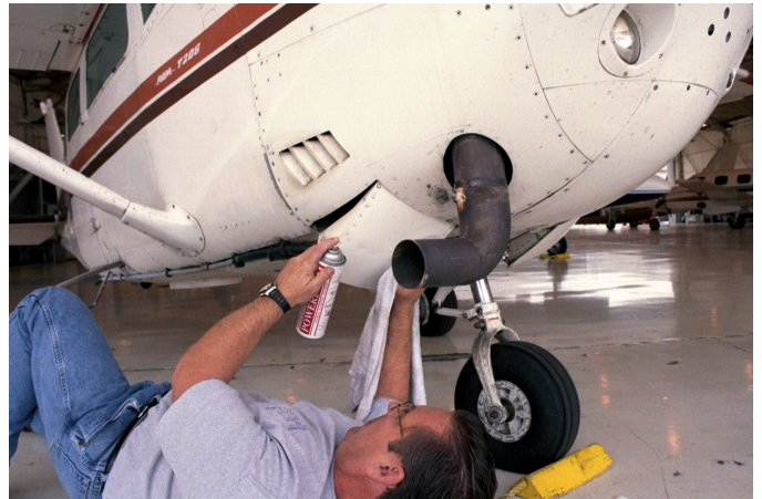
Use Powerfoam or BIO-JET to clean belly on Cessna 206
