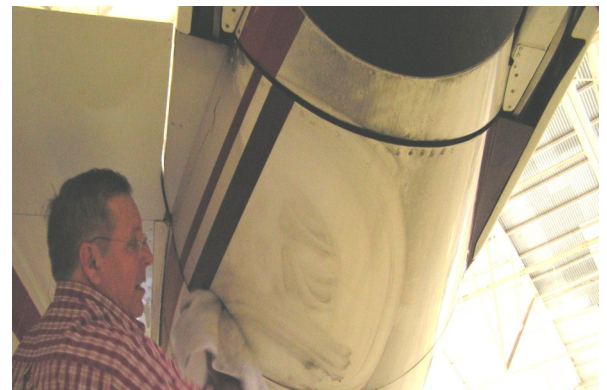
Powerfoam is our choice to clean the bottom of dirty engine nacelle on a Hawker 1000.
