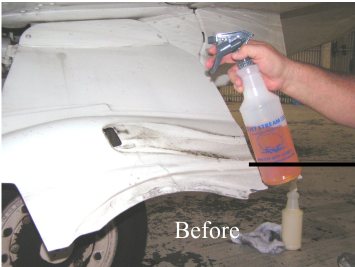
Using Bio Jet to remove heavy accumulations of hydraulics from the gear door of a Hawker 1000.
