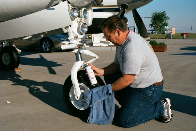
Using Powerfoam to clean bugs and grease from nose gear of King Air 200.
