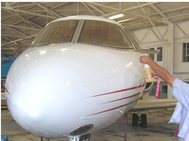
Using Quick Turn to clean bugs and dust from the fuselage of a Hawker 1000.
