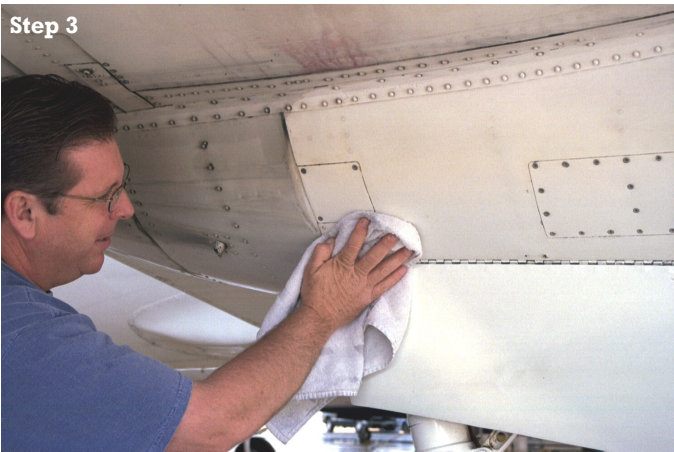
Three simple steps using Powerfoam when cleaning carbon and oil from gear door and bottom of cowling on King Air 90.
