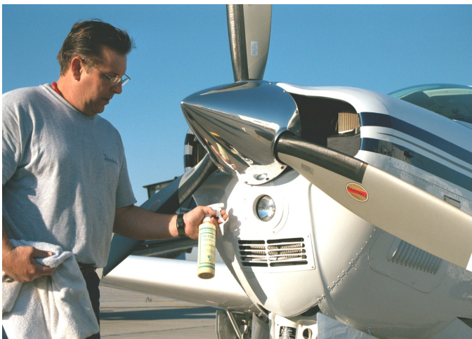
Using Flyers Speed Wax to remove bugs from nose of A-36
