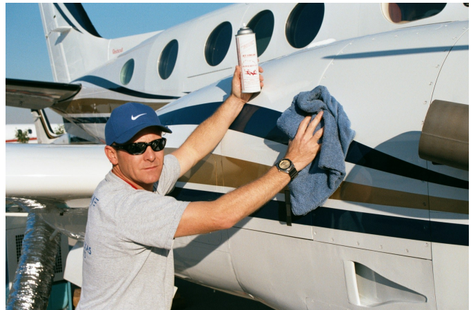
Using Powerfoam to clean carbon and oil from a King Air 90 engine cowl.
