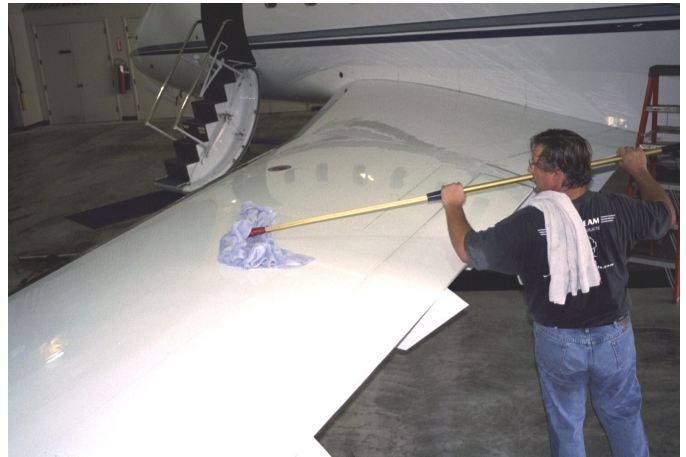
To remove dust from the top surfaces of aircraft when dry washing, use a towel wrapped around a squeegee. Spray the top of wings with Quick Turn , it will help the towel pick up dust from surfaces of aircraft.
