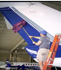
**Aircraft Clean Up:** Buffing metal makes quite a mess. Wool buffing pads will give off a black wool fuzz that will cover the aircraft and hangar floor. You will need to dust off the aircraft using a towel wrapped around a squeegee as shown in picture on left. If you will not be cleaning the aircraft after polishing the brightwork, we recommend covering the aircraft with plastic or paper before buffing.
