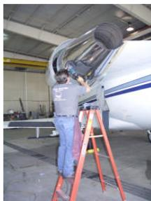
**Polish Leading Edges On Tail:** You will need a scissor lift to reach the vertical and horizontal leading edges on the tail of the aircraft. Most flight departments that operate the
