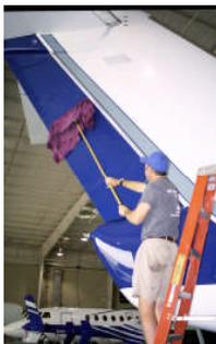
Wool buffing pads will give off a black wool fuzz that will cover the aircraft and hangar floor. You will need to dust off the aircraft using a towel wrapped around a squeegee as shown in picture on left. If you will not be cleaning the aircraft after polishing the brightwork, we recommend covering the aircraft with plastic or paper before buffing.
