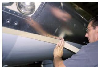
**Step 1: Taping:** Using 3M two inch masking tape, part # 2311, tape all painted surfaces adjacent to metal being polished. Taping will protect the painted surfaces from black polish residue that forms when polishing metal.
