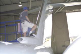
extreme caution when operating the scissor lift around aircraft. We recommend using a spotter below the lift when positioning the lift next to an aircraft. When polishing the bottom section of the vertical leading edge, you will be required to stand on top of
