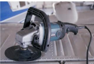
**Polisher:** Use a variable speed buffer like the Makita model #9927C. This buffer is light weight and has a rpm range between 800 and 3000. It has plenty of power and will not bog down. The variable speed will allow you to slow the buffer down and safely
