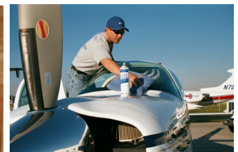
Using Plexi-Clear to clean the front windscreen on A-36 Bonanza.
