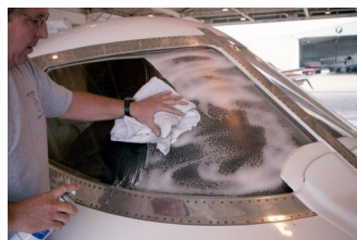
Using Plexi-Clear to clean cockpit and instrument panel in Hawker 800.
