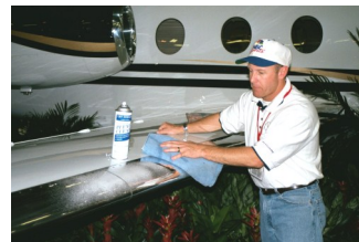
Using Plexi-Clear to clean bugs off polished aluminum. Plexi-Clear will not dull polished aluminum.
