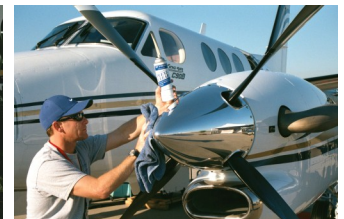
Using Plexi-Clear to clean bugs off polished aluminum. Plexi-Clear will not dull polished aluminum.
