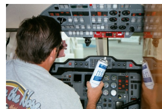
Using Plexi-Clear to clean cockpit and instrument panel in Hawker 800.
