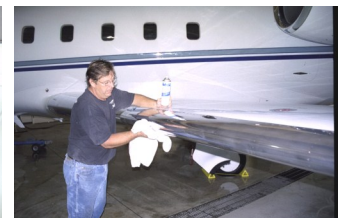
Using Plexi-Clear to clean bugs off leading edge of Challenger 600.
